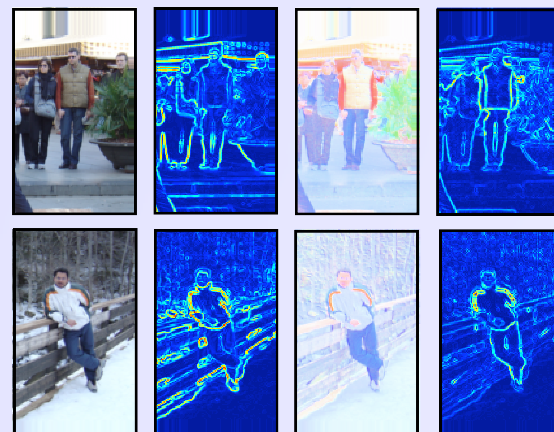
Columns from left to right: (i) original image; (ii) gradient magnitude of original image; (iii) color normalized image; (iv) gradient magnitude of normalized image.
